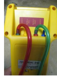
Green hose goes to outside; red to flue or under door.
